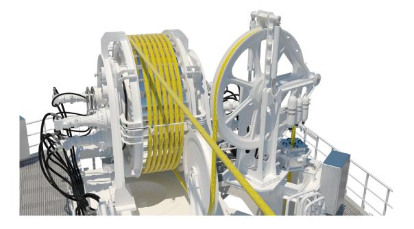
The capstan consists of two interlocking drums slightly angled and offset to each other.
