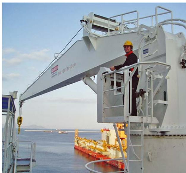
Applications: Safe, reliable handling of spares and provisions on all type of vessels and for handling free-fall boats.
