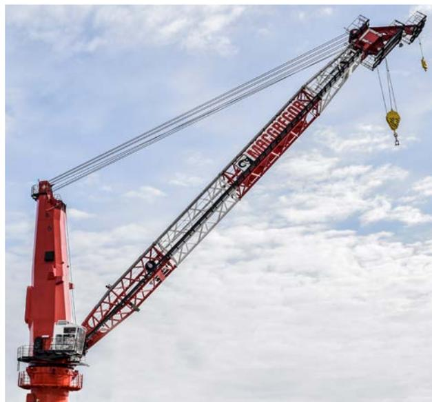
Applications: designed for installation on floating or fixed platforms. Heavy offshore operation in compliance with the 7th edition of API-2C.
