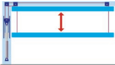
Jigger-winch mounted in the side shell structure
