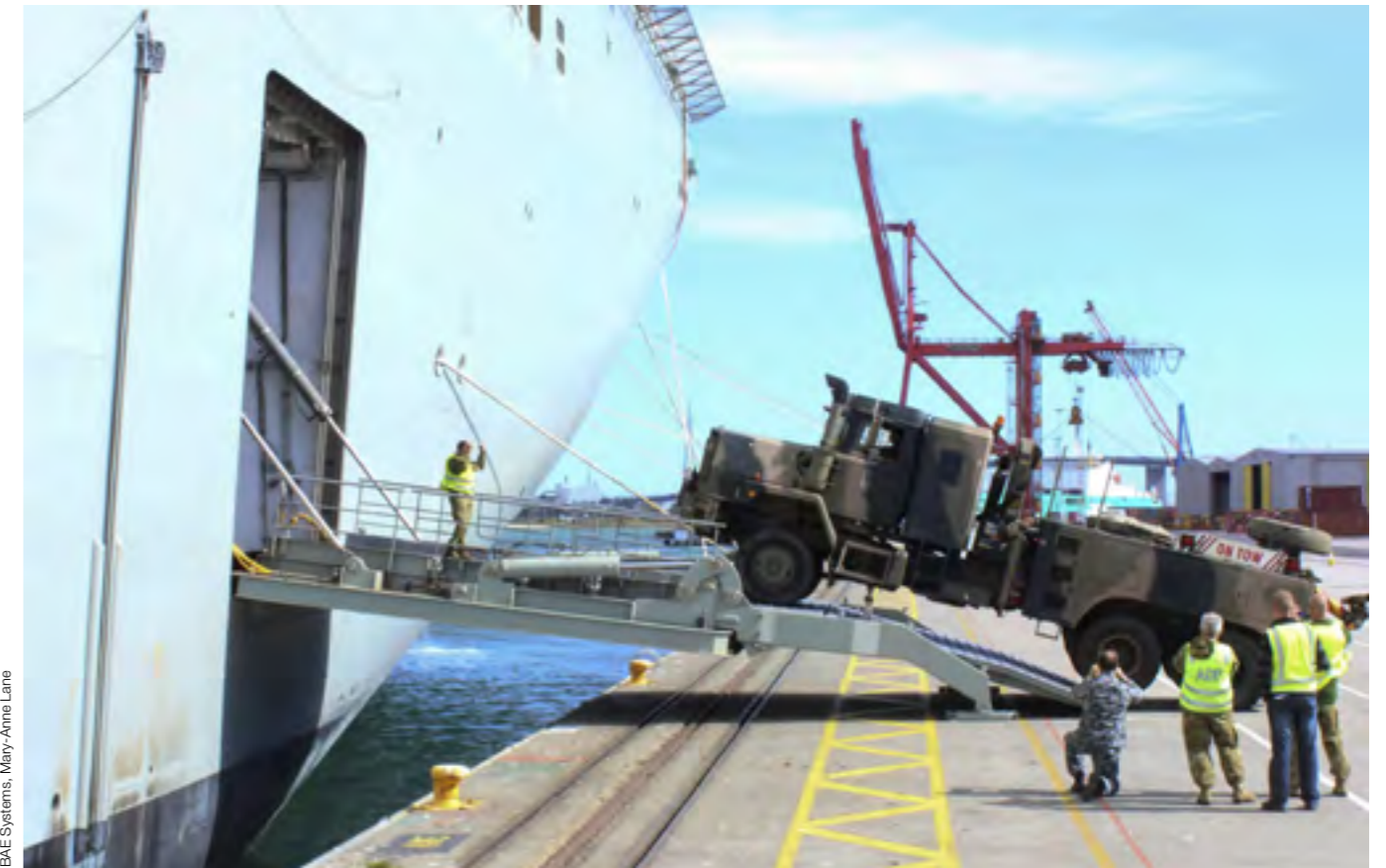
The side ramp on board Landing Helicopter Dock (LHD) HMAS Canberra that provide access for 65-tonne vehicles
