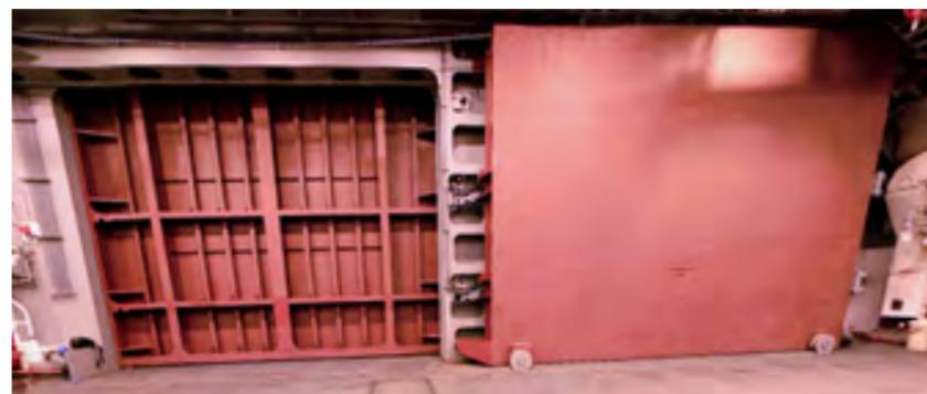
Robust and reliable sliding bulkhead doors have been fitted onboard RFA Argus. They incorporate innovative technology and are developed from proven designs.
