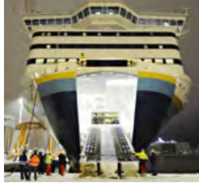
The new bow ramp has a clear driving width of 3,5m and is coated with Bimagrip to prevent vehicles from skidding.
