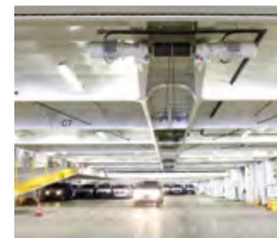
possible to feed power back into the ship's power supply when larger winches, such as those found on quarter ramps, lower heavy loads.
