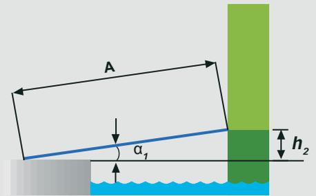
Fig. 3: Light ship during high tide
