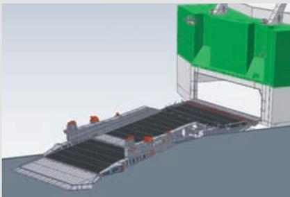
Fig. 1: The main section functions as a watertight door
