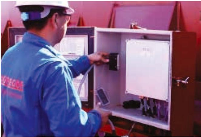
**PREPARING FOR OPERATION:** Connecting the portable operation unit to the control box.
