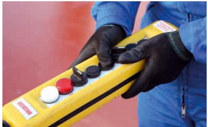
**OPERATION:** The portable operation unit allows the operator to move freely around the coaming to observe and control the operation from wherever is most convenient.
