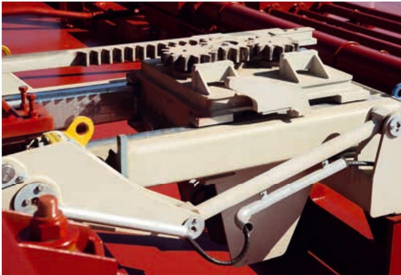
MacRack employs a combined rack-and-pinion drive and lifter system that makes separate hatch cover lifters obsolete. Electric operation removes the need for hydraulic pipework and other components.
