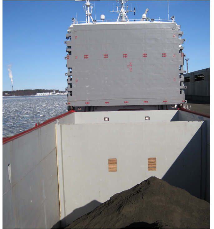
Movable bulkheads are typically operated by connecting them to weather deck folding hatch covers, or by ship or shore cranes. The bulkheads are locked into position either by manually or hydraulically-operated pins. They can be placed at several locations depending on the cargo hold design.
