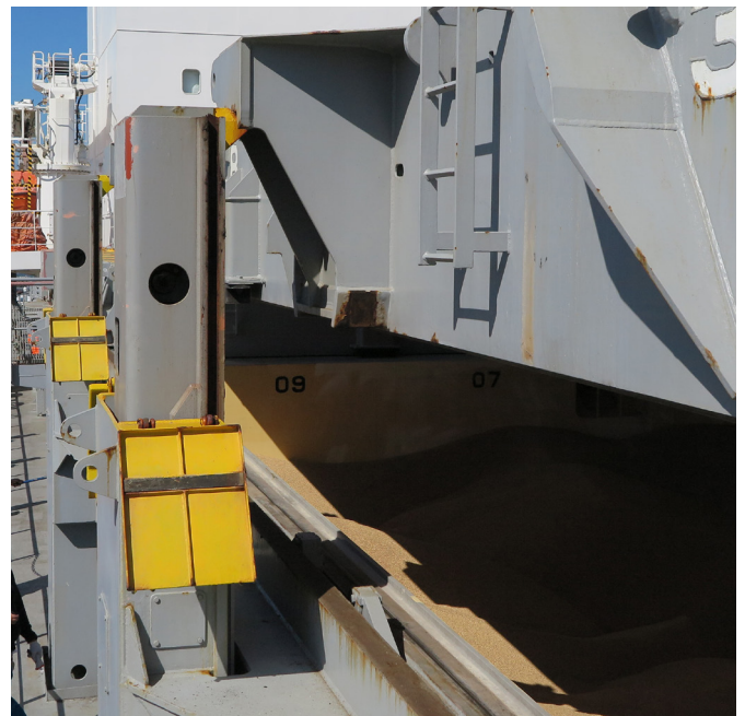
The hydraulic cylinders lift the high-lift panel to accommodate the rolling panel underneath it
