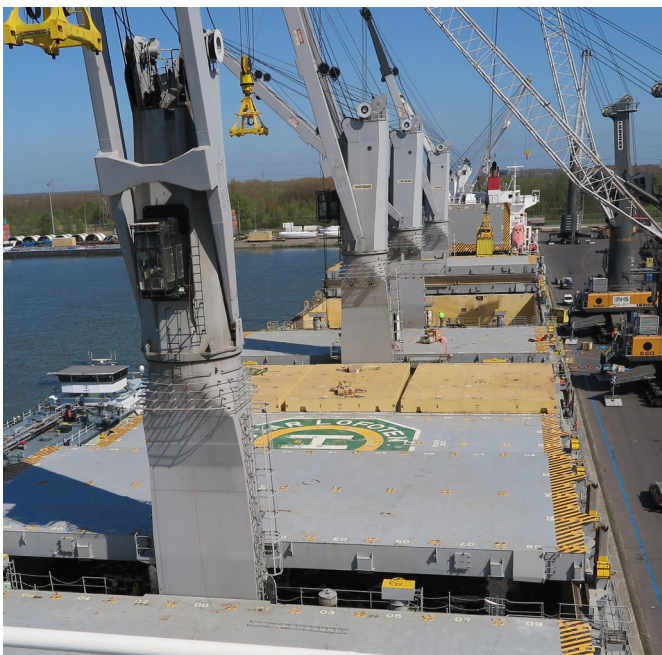
Piggy-back hatch covers are used on ships with limited deck space
