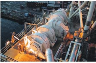
MacGregor anchor windlass for a 145mm chain on board the *Snorre B* production platform in the North Sea. The windlass consists of four cable lifters with a single electric drive/gearbox and two fail-safe band brakes per cable lifter. Brakes can be released using stored energy (accumulator) in an emergency situation.
