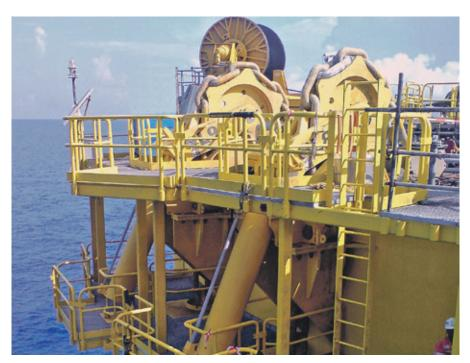
MacGregor Roller RamWinches on board Shells's *Perdido Host Spar*. The nine chain jacks are arranged in three equal groups along the top circumference of the hull. Stalling capacity of each chain jack is 725 tonnes.
