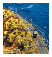
MacGregor RamWinches on the *Devil's Tower* spar platform in the Gulf of Mexico at a depth of 1720m.
