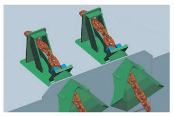
The MacGregor bellmouth chain stopper provides a simple means of chain holding in benign areas where the mooring line can run straight off the deck. The stopper is designed for the full breaking load of the chain. In addition, a mobile tensioning device has been designed to move from stopper to stopper. A portable hydraulic power unit can be delivered to power the tensioning device.
