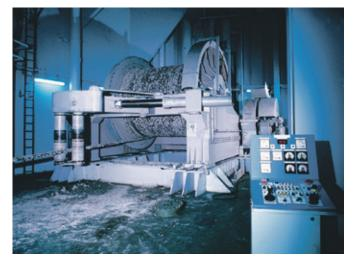
MacGregor wire winch on the crane barge *Saipem* 7000. This is the largest mooring winch drum MacGregor has designed and manufactured to date. The drum can accommodate 3000m of 96mm wire.
