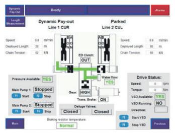
Graphic display built into an operation panel for MacGregor Windlasses installed on the *Aker Barents* drilling rig. Each windlass is driven by a 450kW electric AC motor. The hydraulic power units (HPU) are of a state-of-the-art design that provides a dependable source of power and performance in harsh and varying offshore environments. High-pressure hydraulics in a "ring main" system enables use of smaller pipe diameters and shorter pipe lengths.
