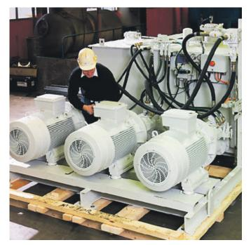
A typical high-pressure hydraulic power unit with three pumps. The cooling of hydraulic oil can be done via seawater, freshwater, or an air system.
