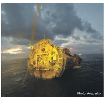
MacGregor RamWinches installed onboard the *Lucius* spar platform. The winches are designed to endure submerged conditions prior to upending.
