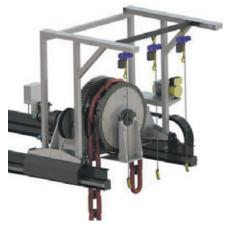
The movable windlass is a concept designed to operate multiple mooring lines within the same area. Normally, one windlass skids along a special foundation to operate one mooring line at a time.
