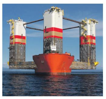
*Blind Faith* semisubmersible being transported to the Gulf of Mexico where it was installed in 2008. MacGregor RamWinches and chain fairleads for 127mm R4S chain were installed at the yard in Norway before sail-away.
