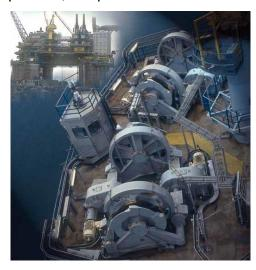
**1997:** Development / Introduction of the Pusnes RamWinch, an on-vessel mooring winch designed as an alternative to conventional rotating winches.
