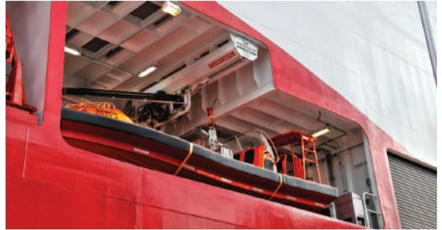
We can supply a robust **G-type** davit, especially suited for operations in rough conditions. Our **T-type** davit has a compact design which allows for installation in hangar with limited height and/or depth. The space-saving design of this telescoping davit leaves the vessel deck and bulkhead clear, supporting the davit only by the overhead ship's structure. MacGregor **A-type** davit is a cost-efficient alternative that offers proven performance and reliability.
