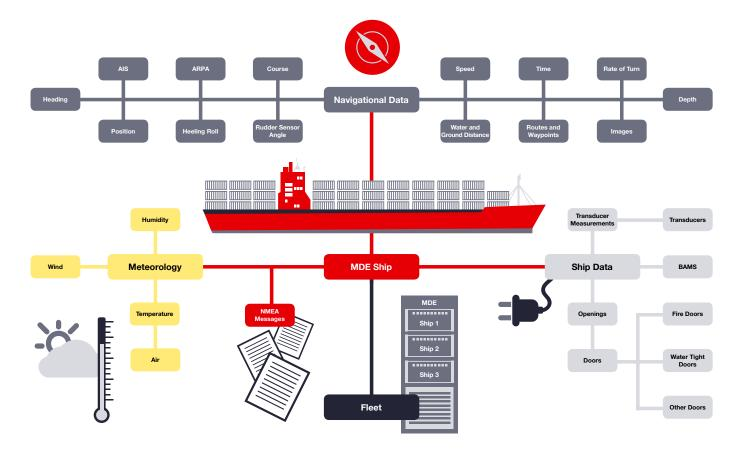
MDE was developed inhouse by MacGregor's Interschalt and generates a real-time process picture in the form of a data tree of your ship or fleet for further use on land. The standardised, uniform and bundled data cloud produced in this process can be used to perform such jobs as risk analysis.
