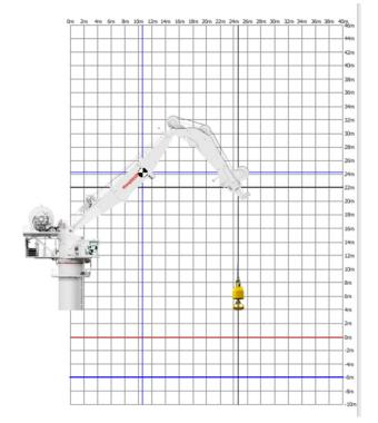
Parameters for any operation may then be entered, and you will get the corresponding load curves and crane view for input to your lifting procedures. The results may be printed.
