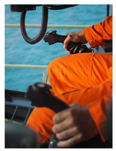
Operations to a greater depth often require the operator to hoist or lower the winch at a defined constant speed over a long period of time.
