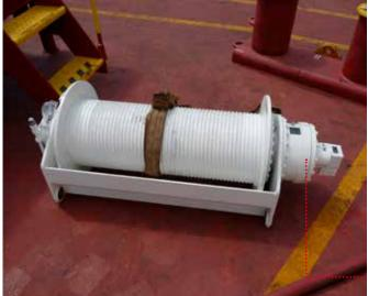
To handle personnel, cranes need to be updated with new parts. A MacGregor personnel handling system installation includes a winch with double brakes, valves, hydraulic hoses and various other components. MacGregor liaises with classification societies to ensure that each element meets approval before installation and testing.
