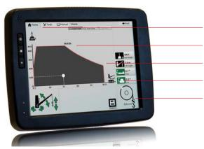
Real-time information on active systems Load/speed/outreach information Logs information for analysis Errors/warnings/events Touchscreen display
