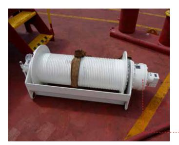
To handle personnel, cranes need to be updated with new parts. A MacGregor personnel handling system installation includes a winch with double brakes, valves, hydraulic hoses and various other components.
