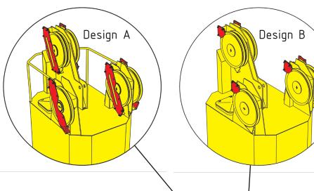
MacGregor wire sheave guards protect wire-rope sheaves from damage and minimize the risk of them breaking away from the crane.
