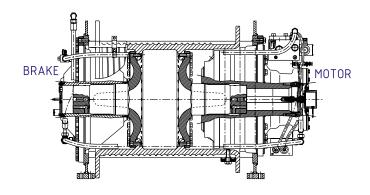
New winch with gearbox and high-speed motor
