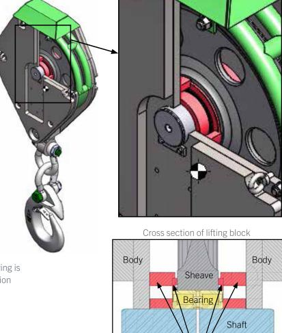
Bearing support kit on both sides of bearing
