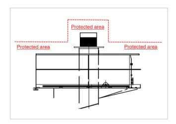
So, how does the system work? As you can see from the illustrations here, we simply combine a slewing range limitation along with a luffing range limiter for the critical area. This effectively is a small amount of hardware that is a very cost-effective solution because it provides an economical alternative to expensive repairs. The system can be tailored to meet all type of cranes and ship board applications.
