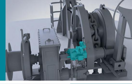
Heavy sea conditions, operating error and other negative influences can make heaving the anchor especially difficult. Overtension on the chain can cause the windlass to go into overload. Overload on the windlass can lead to hydraulic motor damage and be a safety hazard.
