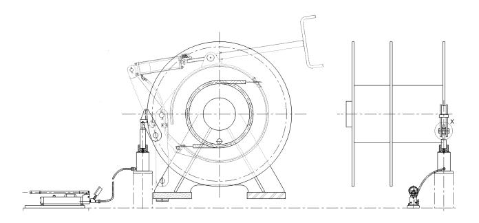
Over time, the brake linings on the drum band brake can start to wear down. This affects the holding capacity and the performance of your equipment.
