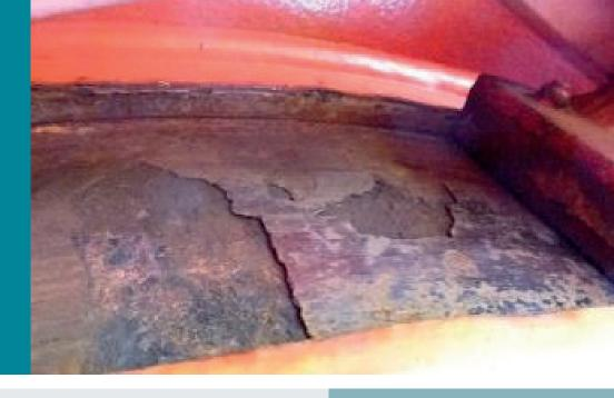
Due to exposure, lack of maintenance or other factors, the metal on the brake ring can begin to corrode and break down. This affects the brake holding force and the life of the product.
