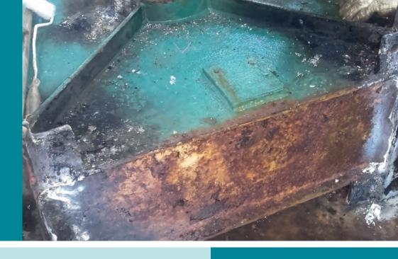
The gear cases are vital to the function of TTS winches but are also constantly exposed to the elements. This can take its toll on the gear case material, causing corrosion. This breakdown and rust usually occur on the underside of the gear case - a spot difficult to reach.
