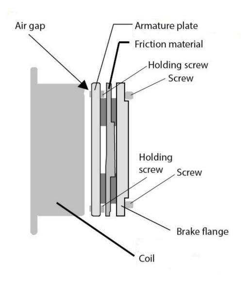
Figure 1: Electro-magnetic brake
