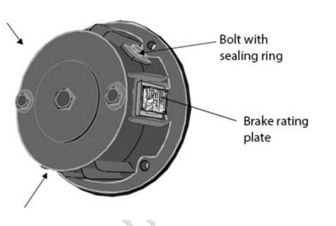
Figure 2: Bolts placed around the casing
