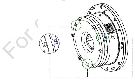
Fig. 10 - Loosen emergency release screws
