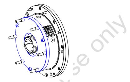
Fig. 8 - Fasten emergency release Allen socket screws
