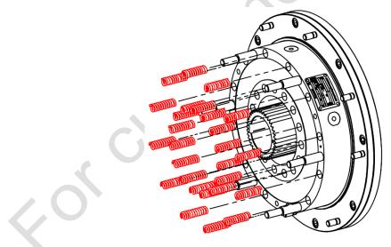
Fig. 7 - Insert new springs
