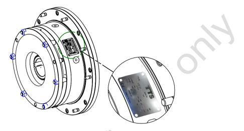
Fig. 9: Coil body nameplate
