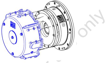
Fig. 2 - Remove the cap
