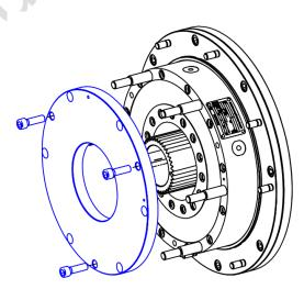
Fig. 5 - Remove armature disc
