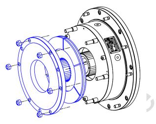
Fig. 4 - Remove brake disc and friction disc
