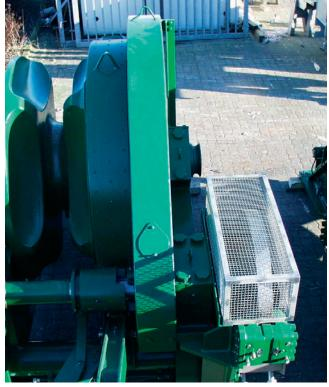
Because this self-contained winch system has no hydraulic pipe interfaces on deck, this both reduces maintenance costs and minimises risk, for instance oil spillage from flange points or mechanical damage from external impact.
